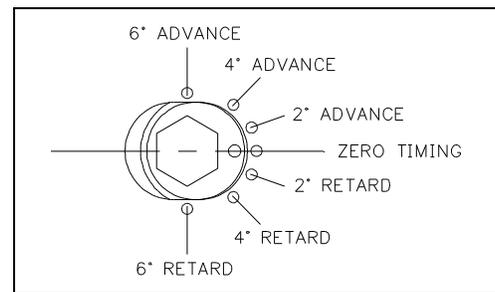
8. **Torque Loose Bolts.** Torque the three (3) Cam Sprocket mounting bolts to 300 in-lb (25 ft-lb).
