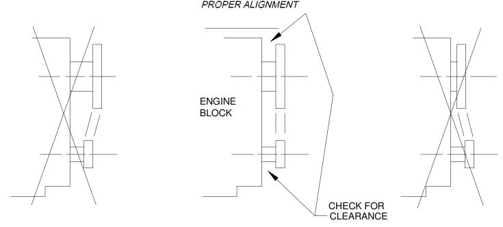
BE SURE TO CHECK FOR CLEARANCE BETWEEN THE ENGINE BLOCK, SPROCKETS AND TIMING CHAIN. CAUSES OF INTERFERENCE COMMONLY COME FROM SLIGHT BLOCK VARIATIONS, WORN CAM THRUST SURFACES, OIL GALLEY PLUGS OR COMBINATIONS OF THE ABOVE.
