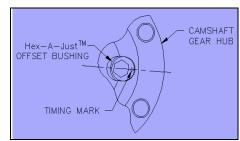
Inserting Offset Bushing (Figure 1)
