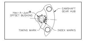
5. Mount the Camshaft Sprocket. Loop the chain over the camshaft sprocket. Align the camshaft and crankshaft timing marks and loop the chain around the crankshaft sprocket. Lift the camshaft sprocket into place on the camshaft, with the **Hex-A-Just**® Bushing in place. Be sure that the timing mark aligns with the crankshaft timing mark. Start the camshaft bolts to hold the cam sprocket in place, but leave the bolts slightly loose.
