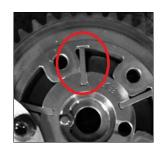
The original equipment (OE) spring actuated vanes produce drag and wear over time.
